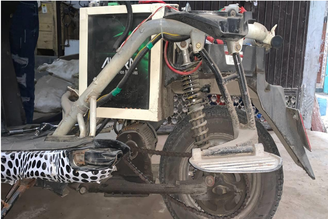
Figure 78 Alterations in Activa for Retro-fit Solution 3
