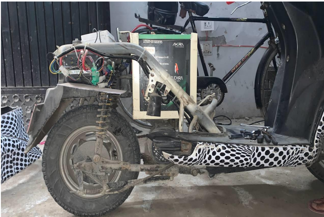
Figure 79 Alterations in Activa for Retro-fit Solution 3
