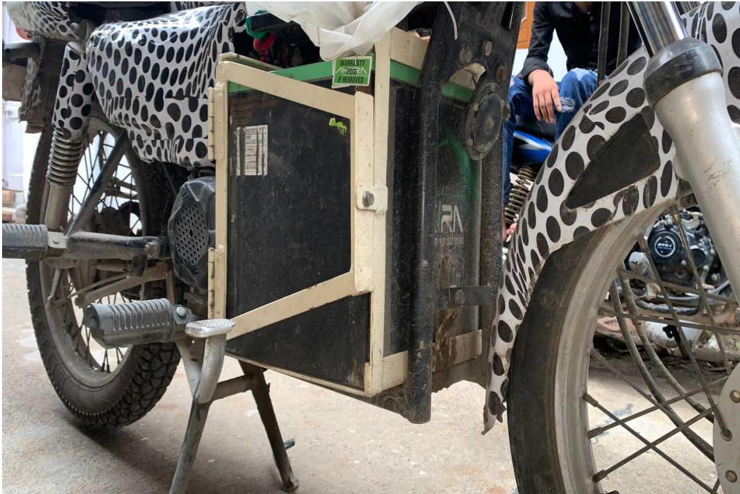
Figure 75 Alterations in Splendor for Retro-fit Solution 3
