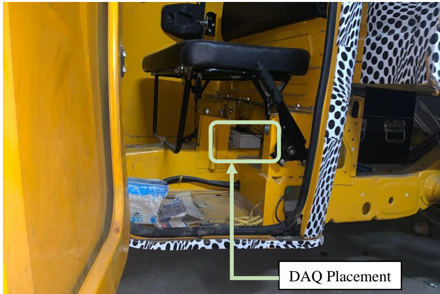
Figure 108 DAQ placement in 3-wheeler cargo vehicle
